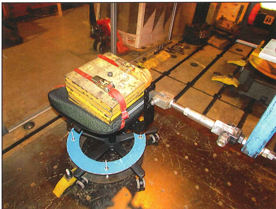
Figure 2 : Tilt mechanism test set-up
